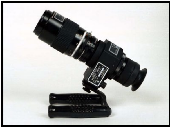
Figure 31: A handheld Cerenkov Viewing Device (ICVD).
