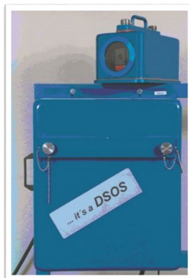
Figure 9: DSOS: Digital Single Camera Optical Surveillance System (courtesy: IAEA, Vienna).
