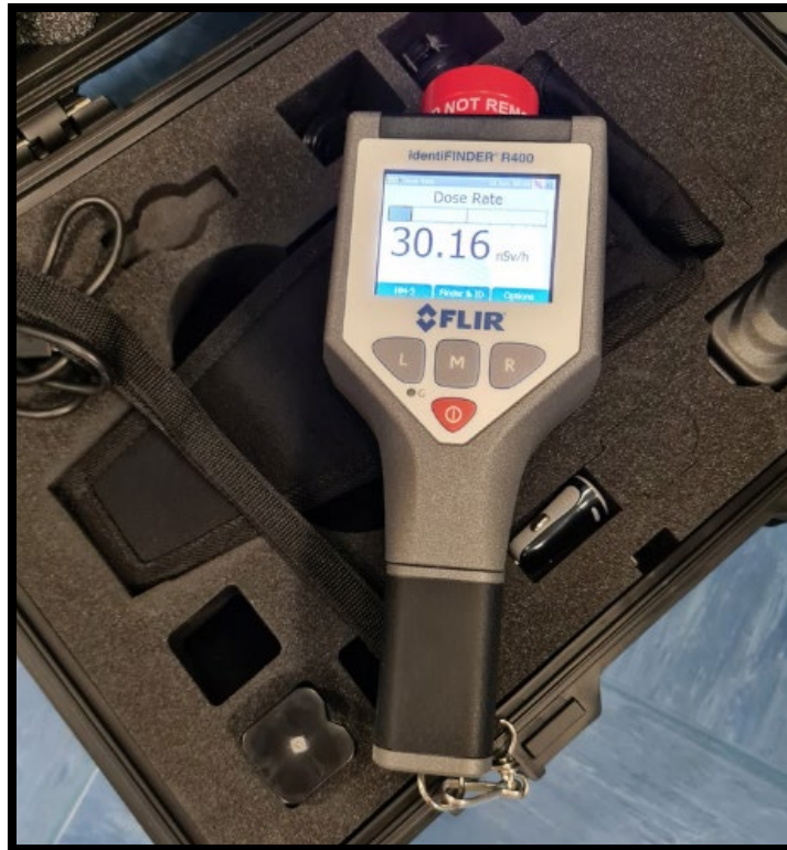
Figure 13: A picture of an HM5 (or Identifinder) used for uranium enrichment verifications. It also measures dose rates. Picture taken in PERLA laboratory, a research and training laboratory of EC JRC Ispra site (Italy).
