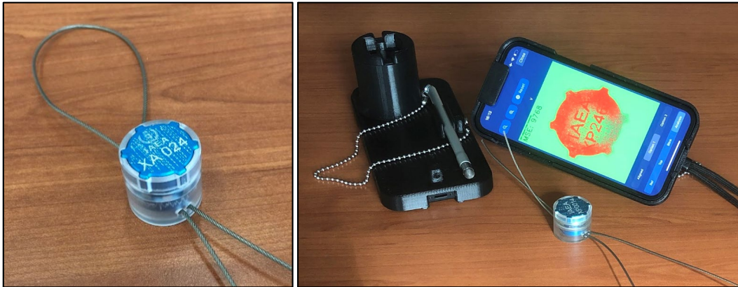
Figure 17: Left: Field Verifiable Passive Seal (FVPS) & Right: FVPS Verifier (courtesy: IAEA, Vienna).
