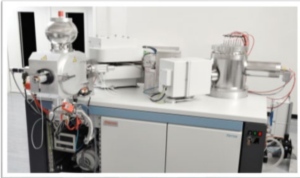
Figure 1: Triton Thermal Ionisation Mass Spectrometer (Thermo Fischer Scientific, Bremen, Germany).
