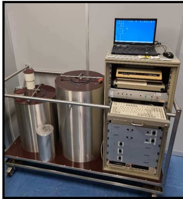
Figure 3: Plutonium air-flow calorimeter used in JRC Ispra made by ANTECH Inc [4].
