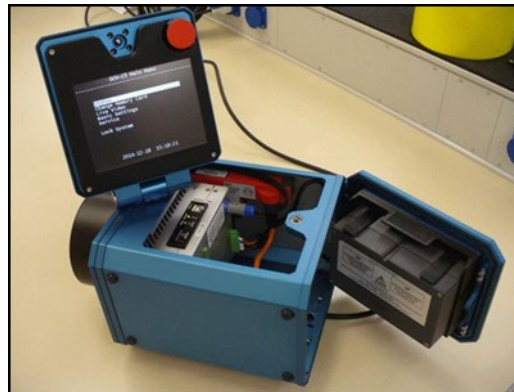
Figure 8: The (open) XCAM with DCD (on top), battery (on open rear door) and AC power supply (red part next to DCM C5) (courtesy: EURATOM, Luxembourg).
