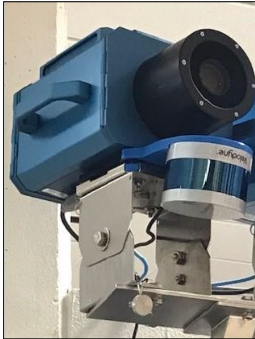
Figure 25: LCCT system combined with NGSS (courtesy: Joint Research Centre, Ispra).
