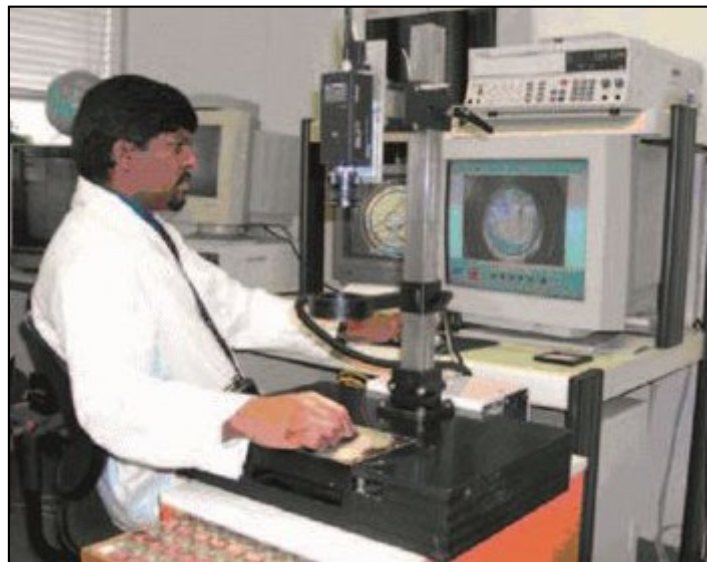
Figure 16: Comparison of metal cap seal images for seal validation (courtesy: IAEA, Vienna).
