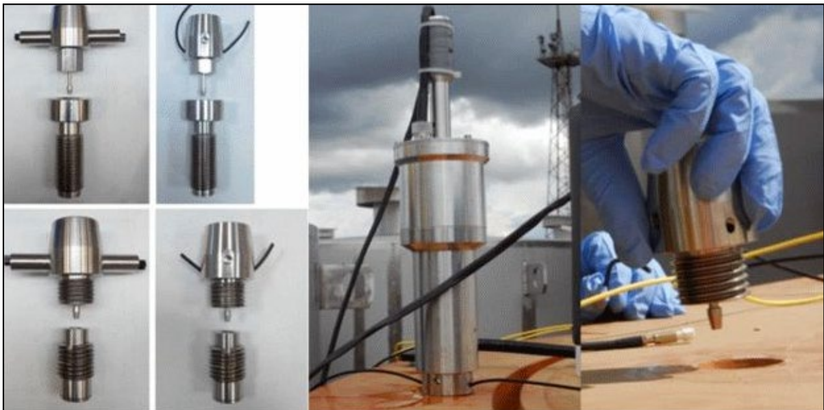
Figure 22: Left: Four different types of UOSBs (Castor, Constor, EOSS & Cobra), center: reading head over the seal, right: UOSB to be bolted on a Constor casks in Ignalina /10/.
