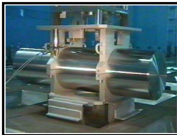
Figure 48: A SMOPY detector. Description of the basic physics: Passive neutron and gamma spectrometry is combined (see the physics description for PG scanning and passive neutron measurements).
