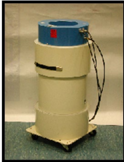
Figure 20: "Los Alamos" High Level Neutron Coincidence Counter (HLNCC).
