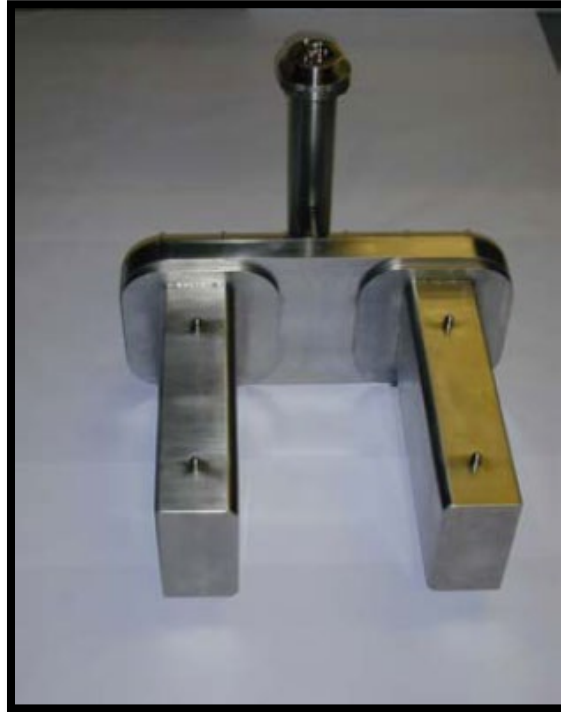
Figure 24: Under Water Coincidence Counters - Model 2106 (UWCC).
