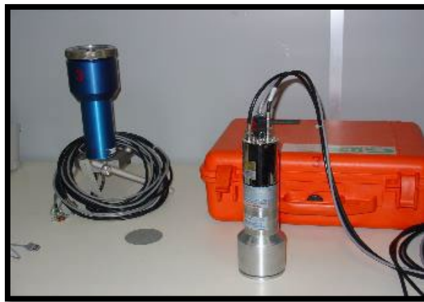
Figure 10: Example of a NaI scintillator used for safeguards inspector trainings in EC JRC Ispra, Italy.
