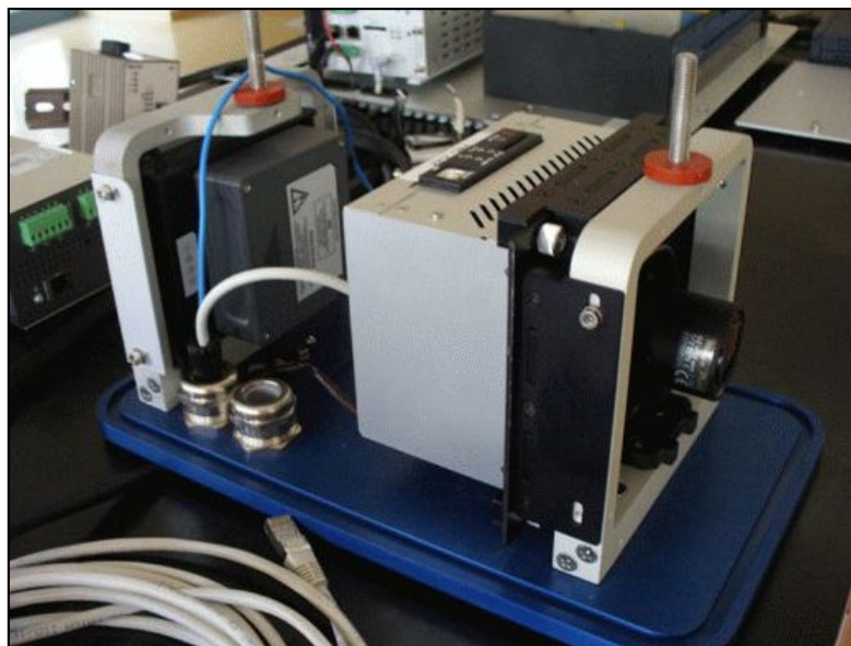
Figure 5: XCOH with DCM C5 with standard lens (fish eye lens with 180 degree angle of view is also mountable) and half size battery mounted in standard blue enclosure (courtesy: EURATOM, Luxembourg).
