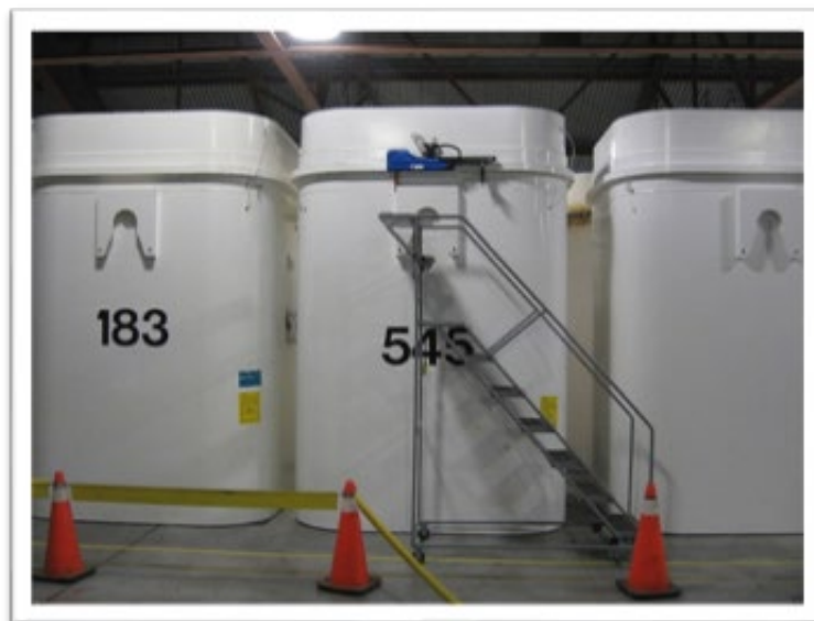
Figure 24: LMCV scanning weld of spent fuel cask (courtesy: IAEA, Vienna).
