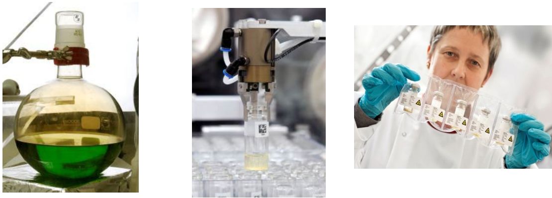
Figure 4: Preparation of U/Pu mixed large-sized dried (LSD) spikes.
