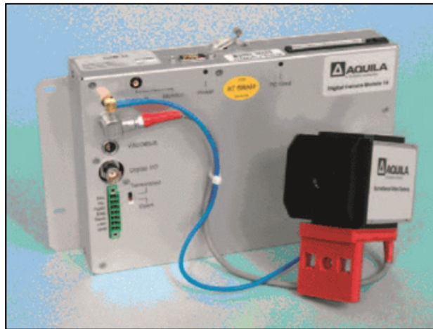
Figure 4: DCM 14 with video CCD camera (Charge Coupled Device) (courtesy: IAEA, Vienna).
